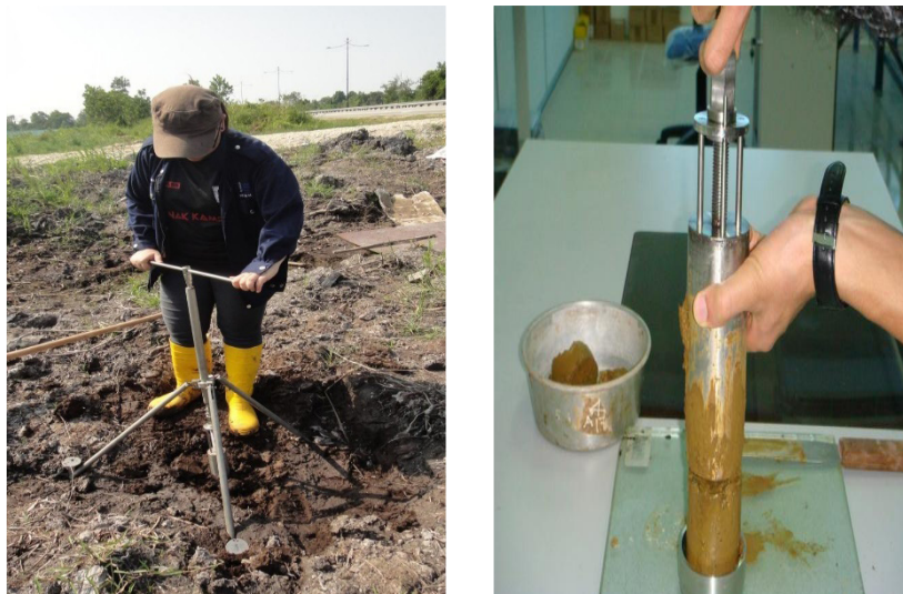
Figure 3 – 5. Tropical peat sampler with built-in extruder
