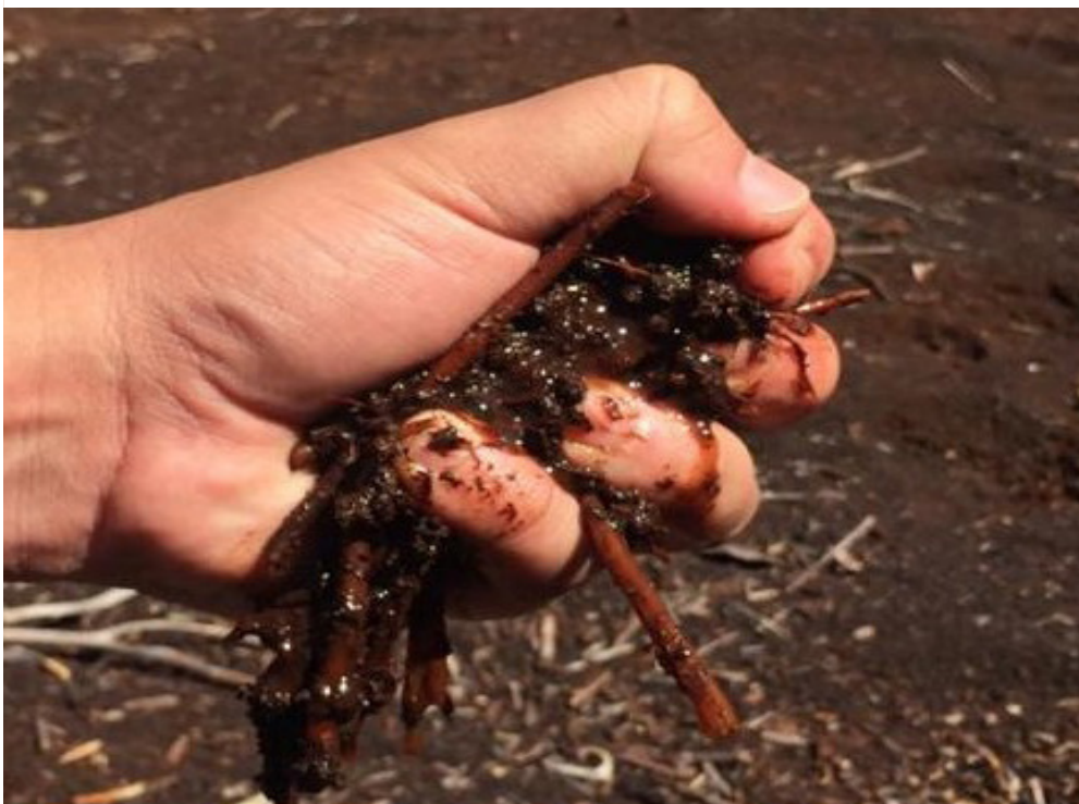
Figure 3 – 8. Peat classification using hand squeezing technique (courtesy photo: Adnan.2019)
