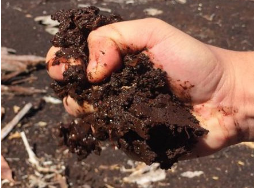
Figure 3 - 2. Peat Decomposition Identification In-Situ (courtesy photo : Adnan,2019)
